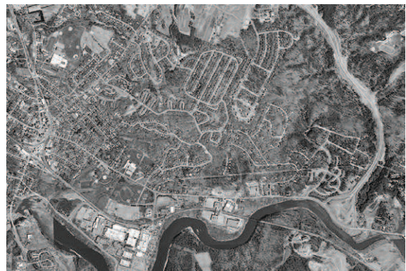
Essex, VT. Sprawl extends roads and drainage channels into areas that were previously disconnected in terms of stormwater. This short-circuiting of natural drainage networks greatly increases the volume, speed, and efficiency of runoff.
